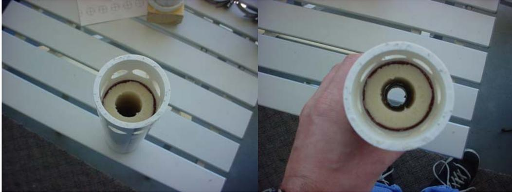
2. The last grain should be even with the “BOTTOM” of the pipe.
