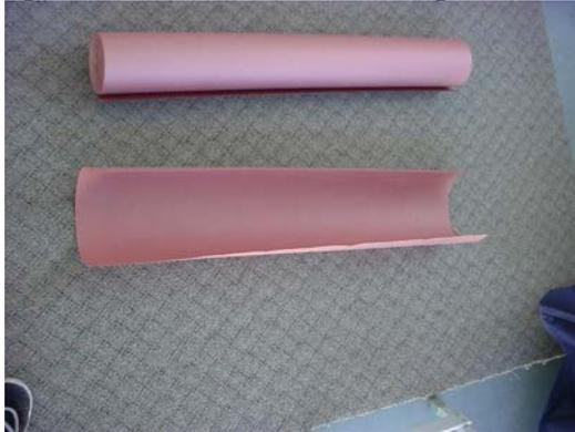
2. Test-roll the strip around a 24" length of 1-1/2" Sch 40 PVC pipe. The straighter the cut on the paper, the straighter the tube will be.
