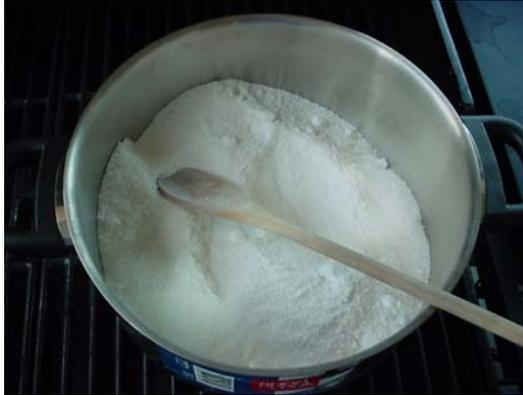
5. Melt this mixture using whatever means that you use, however, I recommend using Dan's set up. He uses a wok that he sets to 300 degrees with wax in it. The wax serves as a way of transferring the heat to the mixing pot. The temperature is controlled by the wok. This setup helps to reduce the possibility of overheating the mix, causing it to self-ignite. **REMEMBER TO KEEP MIXING THE PROPELLANT AT ALL TIMES TO GET A HOMOGENOUS MIXTURE!!**
