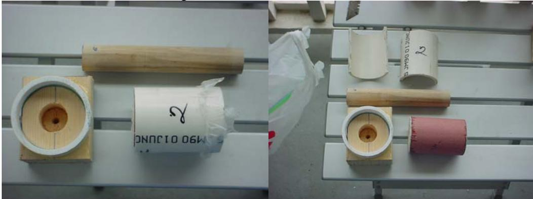
14. Remove the wax paper as best you can from the bore. Don't worry if some still remains, it will be expelled out during motor firing.
