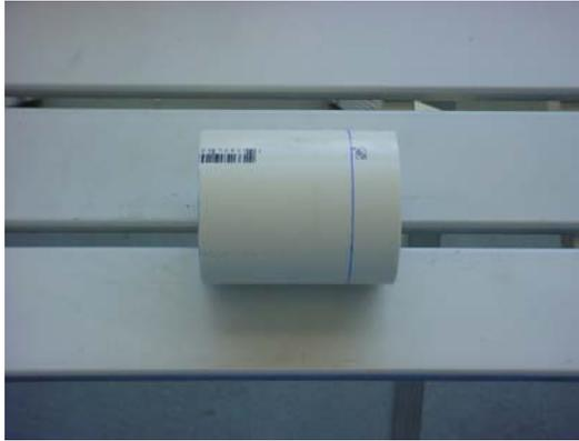
3. Using the hole template provided by Dan from Inverse Engineering, tape the template onto the 3" piece of PVC with the centerline of the holes aligned with the centerline that was drawn around the PVC.
