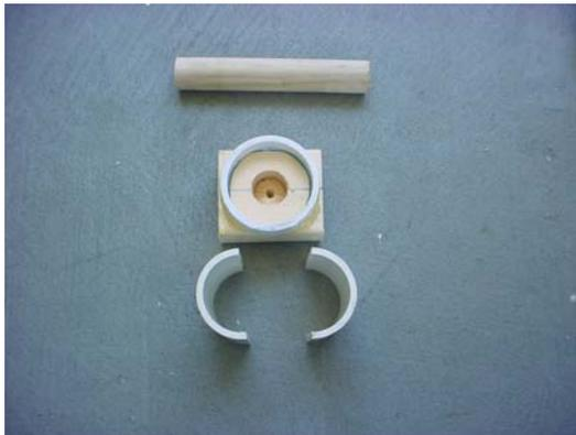
7. Wrap the dowel with one wrap of wax paper and tape it to itself. This helps when you are trying to remove the coring rod.
