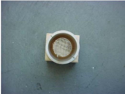
4. Cut a 3" long piece of 2" PVC pipe and cut it in half length wise. This will help aid when separating the grain from the mold.
