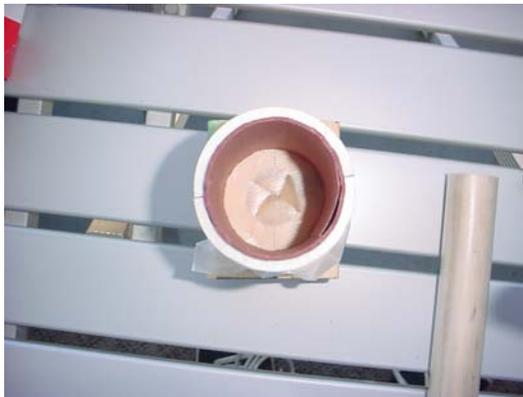
10. Place a completed paper grain tube into the 2" PVC and using the 2 hose clamps, clamp the halves together. (Hose clamps are omitted for clarity.)
