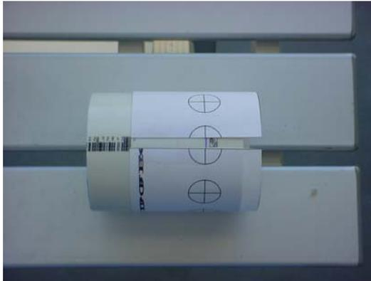
4. Drill out the holes using a 5/8" Forstner bit and remove the template.
