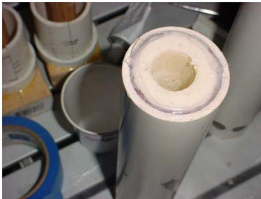
15. Using medium grey PVC cement, glue the 2" coupler/nozzle onto the 2" casing and let dry.
