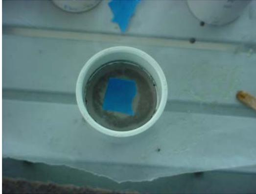
14. Place a bead of high temperature silicone or RTV along the edge where the nozzle and PVC coupler meet. Also place a bead on the "BOTTOM" end of the PVC pipe. This will be used to form a seal between the nozzle assembly and the chamber.
