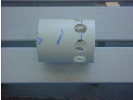
5. Clean up any remaining flashing using a razor knife.
