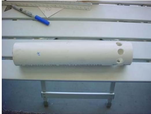
5. Clean up any flashing that remains using a razor knife.
