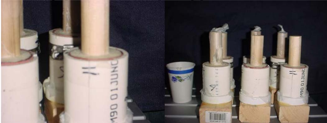
10. Let the grains harden for a few hours before removing them from the molds.
